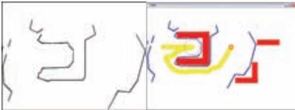
Fig.11 the resulting map created using the line approximation method.
