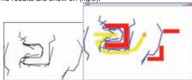
Fig.9. Map of the environment using line approximation
